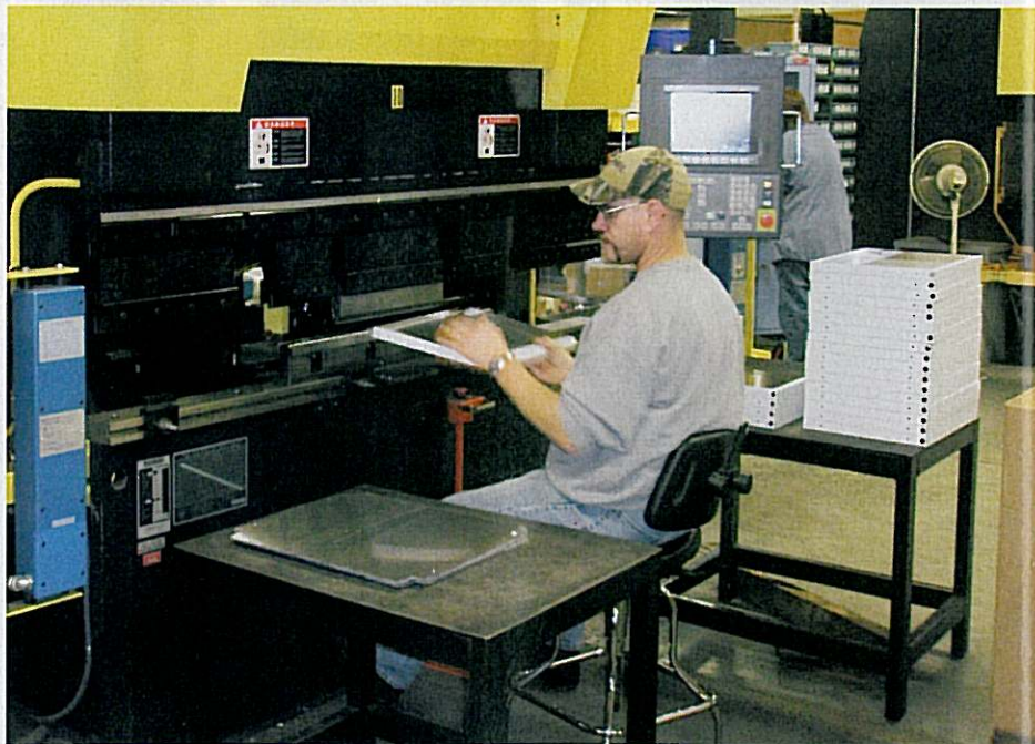
Tom Short operates a new all-electric press brake at Wisco Industries, Oregon, WI. The company employs eight electric and electric-hydraulic brakes, enabling faster, more accurate production with a significant drop in power consumption, as only the control draws power until a brake's foot pedal is depressed.
