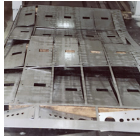
New nesting software helps to fit as many parts as possible on one sheet. These parts are destined for inclusion on heavy-duty equipment.
