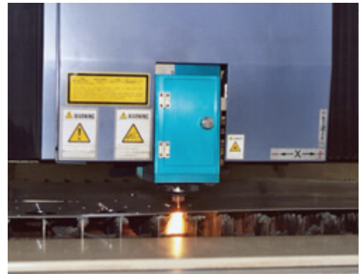
The LVP PLUS laser cutting machine not only is designed to be 50 percent faster than older models, but also features automatic lens focus and height adjustment.
