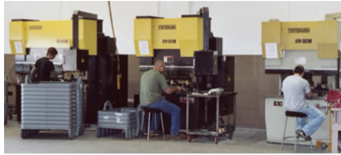
Laser cutting equipment and press brakes go hand-in-hand in a job shop. Approximately 80 percent of the parts that Watson Engineering laser-cuts are bent on three nearby Toyokoki press brakes.
