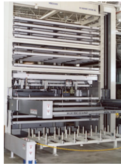
Thanks to the 12-rack material storage tower, laser operators aren't spending as much time on forklifts loading the laser cutting equipment.
